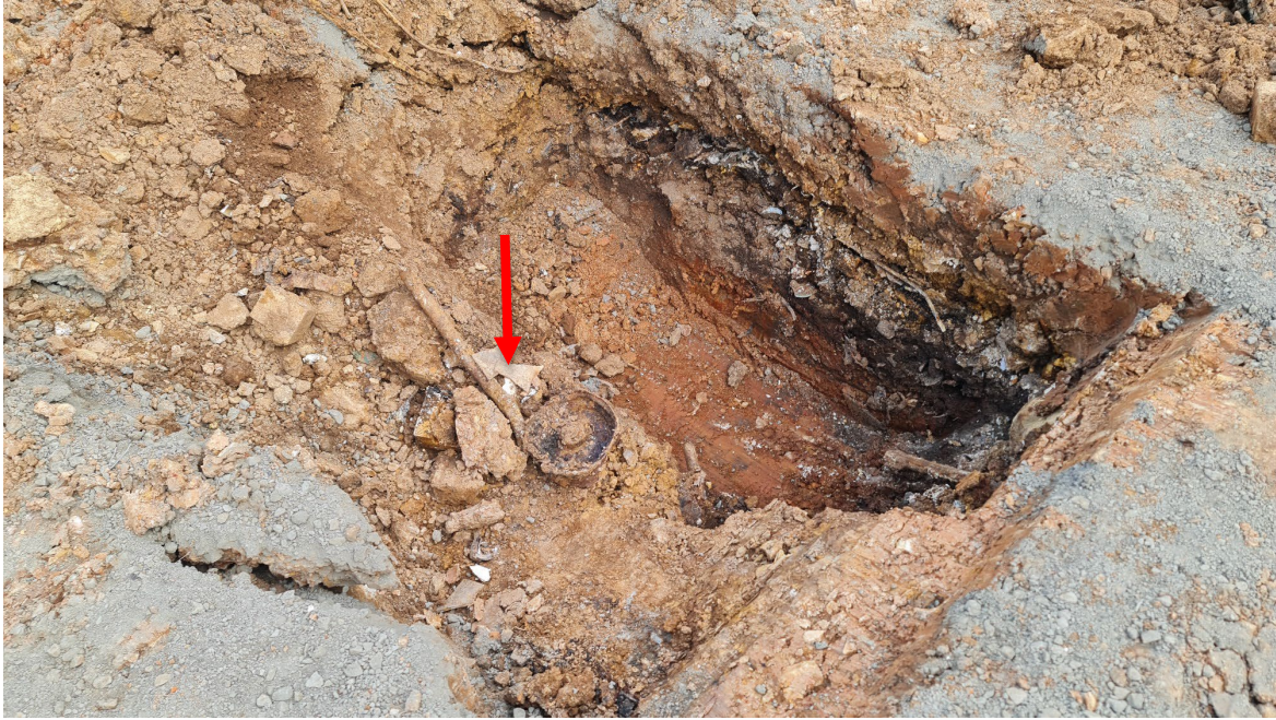
Sandy clay fill soil in former tennis court area containing metal, glass and pieces of asbestos cement sheet debris. Arrow indicates asbestos cement sheet debris
