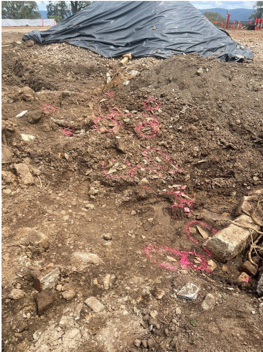
Asbestos cement sheet material found in fill soil near the Medical Centre Building – Contains chrysotile asbestos
