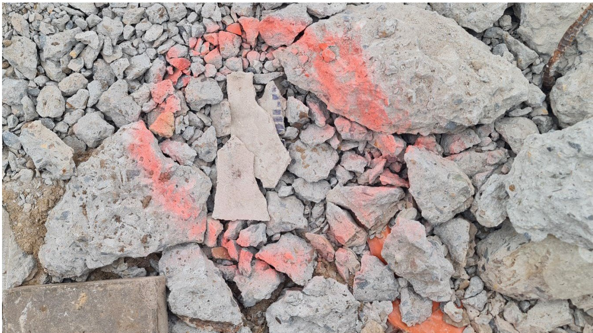
Photograph No. 4: Fragments of asbestos cement sheet identified in fill soil in the chapel area
